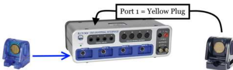
Figure 1. The PASCO 850 Interface and the two types of motion sensors: the Blue motion sensor (plug into PasPort 1) and the Black motion sensor (plug into Digital Inputs 1 & 2)
